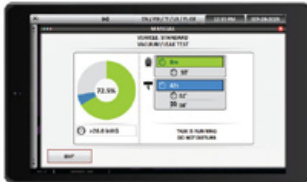
Vacuum/Leak Test Screen fully customizable options allows the user to personalize the times of vacuum and leak testing
