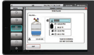
Tank Fill Screen allows for visual, real time progress of tank filling process
